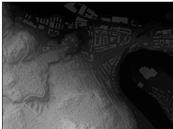
Figure 26: Depressionless DTM after filling the sinks
