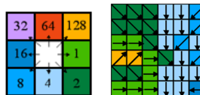
Figure 12: Principle for coding the flow direction in the D8 Algorithm (ESRI 2012B)
