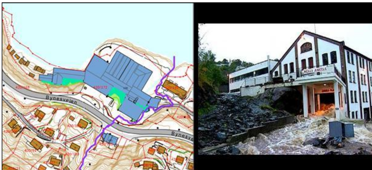
Figure 35: Detail of caution map for flood streams indicating a risk for a building and a picture of a flood stream running through the building on the 22nd of September 2004. (AFTENPOSTEN 2004)
