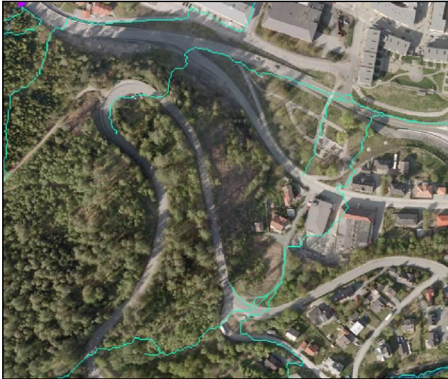
Figure 8: Flood stream (blue) along a road on a steep hill without pavement edges as breaklines. The water leaves the road too early.
