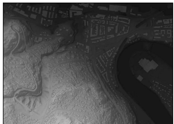
Figure 24: Digital Height Model (DTM) with raised buildings
