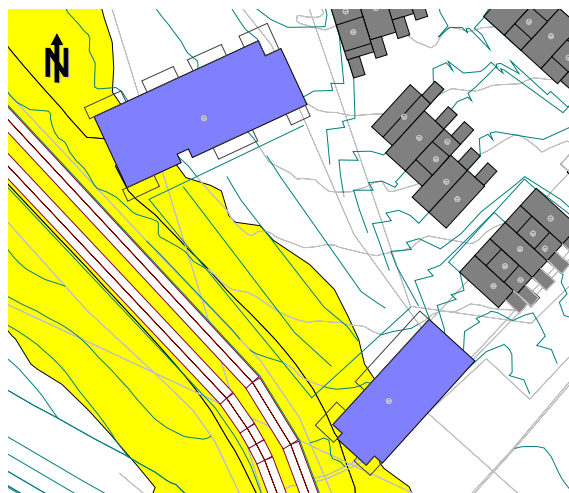
Figur 4-3: Beregnet L_{DEN} 4m over terreng iht. T-1442. Gul sone: L_{DEN} \geq 55 dB. Rød sone: L_{DEN} \geq 65 dB.
