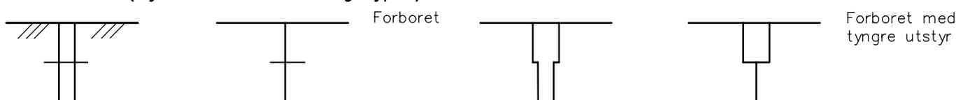
**AVSLUTNING AV BORING (Gjelder alle sonderingstyper)**
